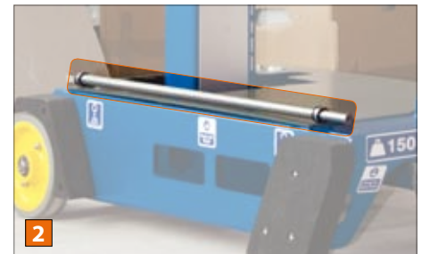
Emergency lowering tool located on chassis
