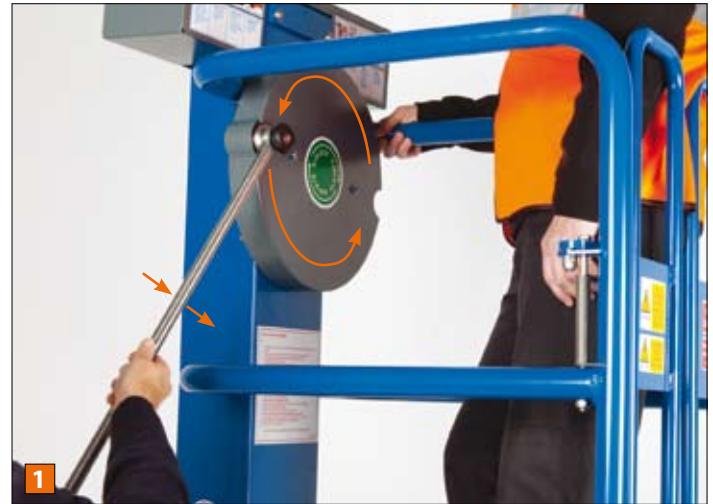
Turn wheel anti-clockwise to bring platform down
